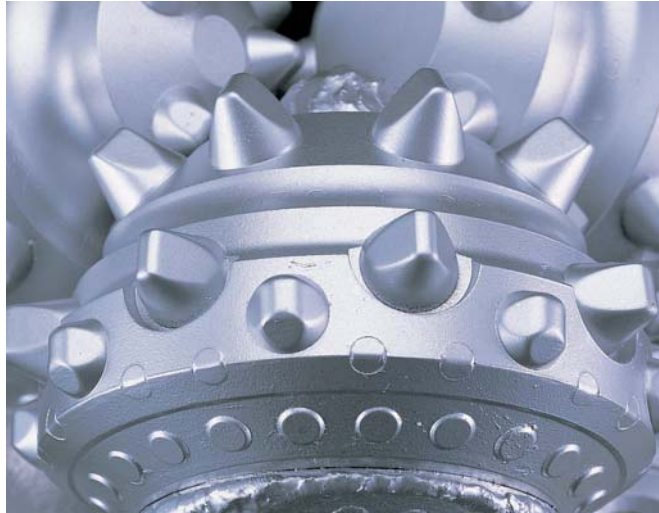
Insert Bits (Ex:8-1/2" X20G F )
